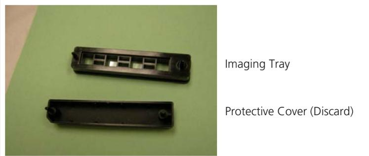
**NOTE:** Imaging Trays should always be handled with care. Do not touch the glass bottom of the tray.
