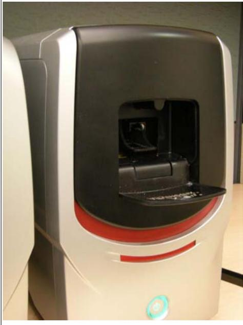
8. Place the Imaging Tray and Array Strip into the Imaging Station (Figure 6.8).
